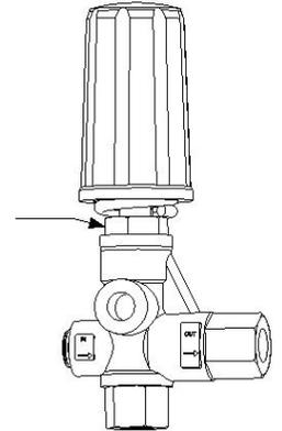
Loosen This Nut To Remove Valve Stem Body.
